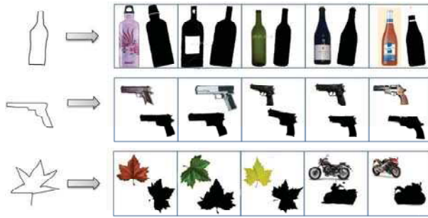
Fig. 2. Queries by sketch: ranked list of similar images based on the submitted queries. For each query, similar image and extracted shape are returned.
